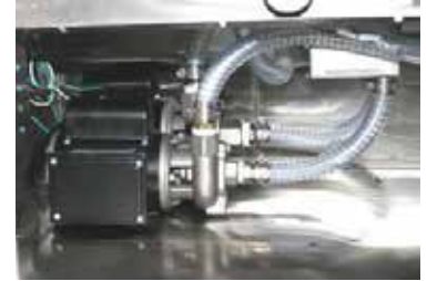
Separate stainless steel wash and drain pumps for quieter operation.
