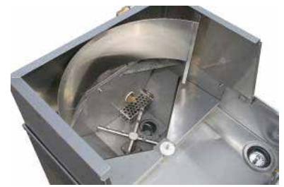
Glassware crossarm with standard spray arm bearing and bayonet pin
